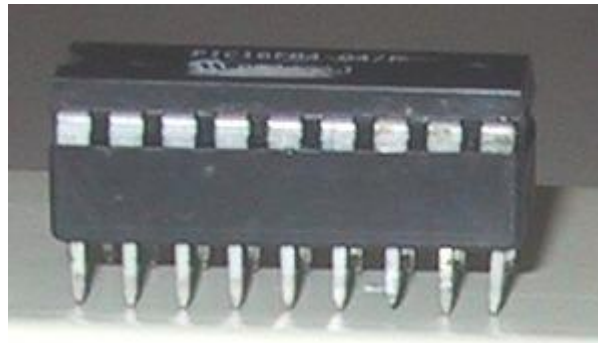
Figure 2: Microcontroller is fitted into an IC base
