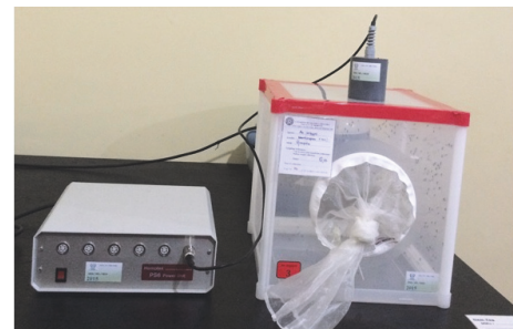
FIGURE 3: Setup of the Hemotek membrane feeding system.
