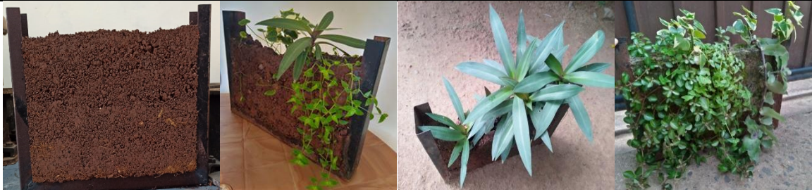
Figure 1: Prepared Slip Form Wall Panels (a) before cultivation, (b, c, d) after cultivation.
