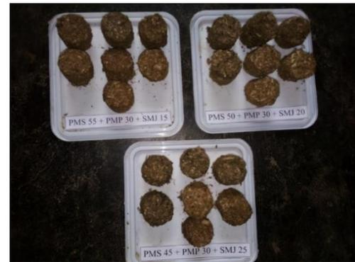
Fig 7. Briquettes used by primary and wastepaper material
