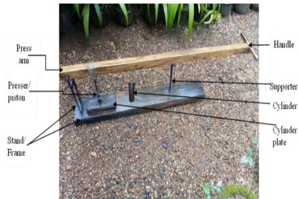
Fig 4. Homemade briquette machine
