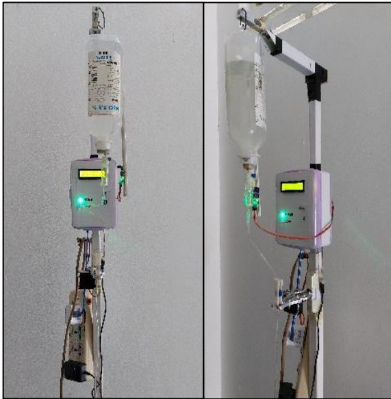
Figure 3: Developed prototype of saline level monitoring system
