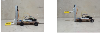
Fig. 7. Lifting up and down process of Forklift
