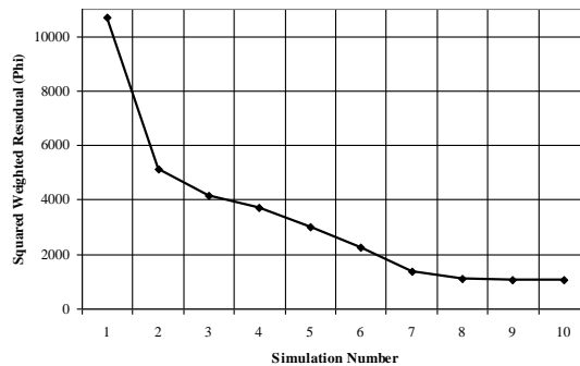
Figure 9 Variation of Squared Weighted Residual with Simulation Steps
